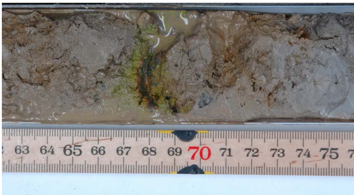
Figure 6.12: An induced fracture observed in KF1 at about 3.5 m b.s. The dark green colour may be due to lower diluted concentration, relative to the more frequently observed red-coloured tracer.
