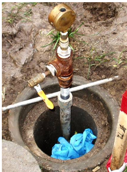
Figur 5.8 Monitering af trykudbredelse i testboring.
